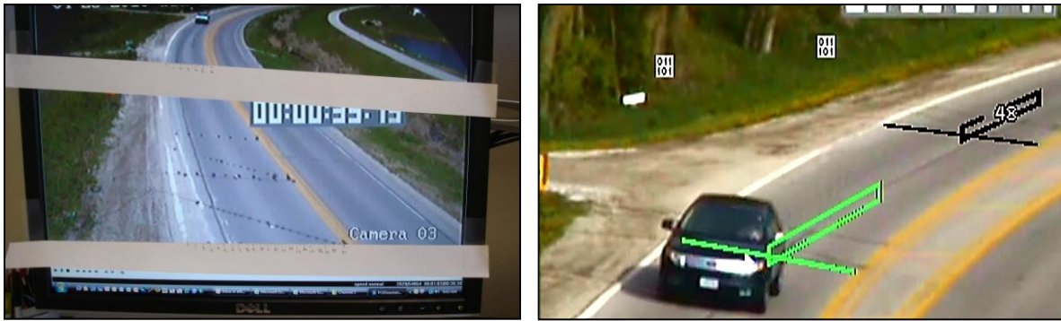
FIGURE 3-4 Manual lateral position reduction (left) and automated speed reduction (right)
