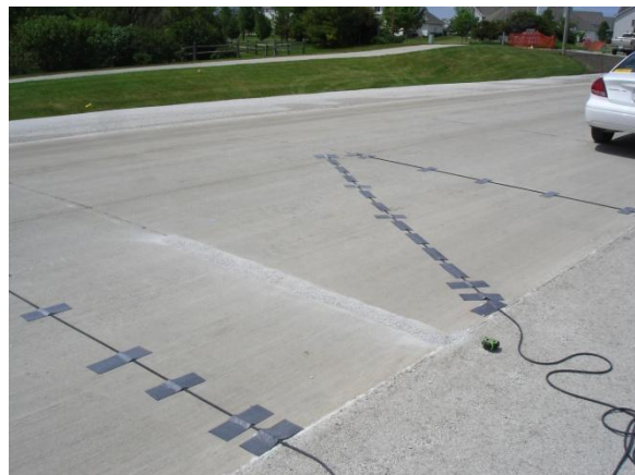
FIGURES F-7 and F-8 Z-configured road tube test bed with limestone aggregate ridge
