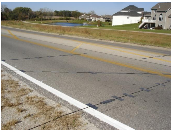
FIGURE G-17 Sta. D z-configured road tubes
