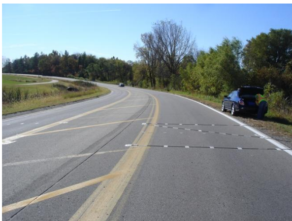
FIGURE G-19 Sta. B z-configured road tubes
