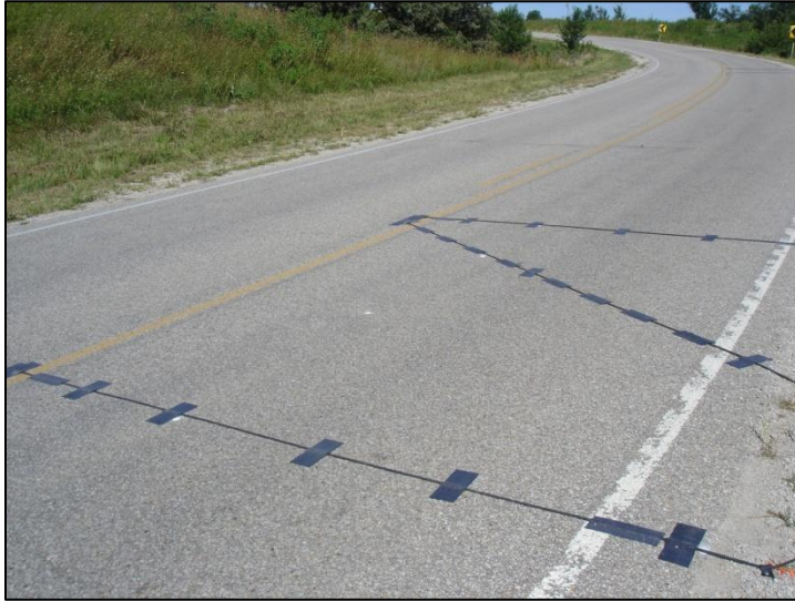
FIGURE 2-9 Pneumatic road tubes setup in a z-configuration
