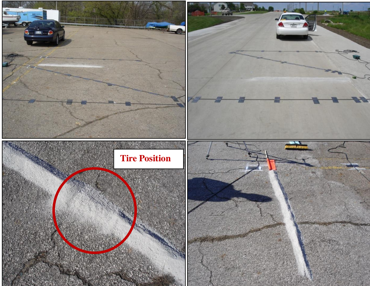
FIGURE 3-2 Closed-course setup (parking lot: top left, city street: top right) and crushed limestone aggregate ridge (bottom left and right)
